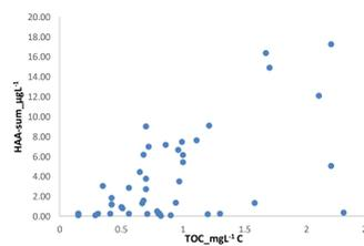
Figure 5. Plot of the total haloacetic acid levels versus total organic carbon levels in Croatia.
