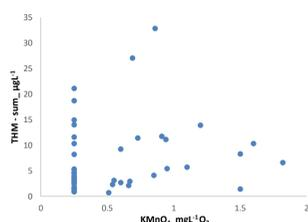
Figure 3. Plot of the total trihalomethane levels versus  $KMnO_4$  levels in Croatia.
