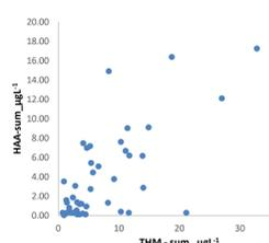
Figure 2. Plot of the total trihalomethane levels versus total haloacetic acid levels in Croatia.
